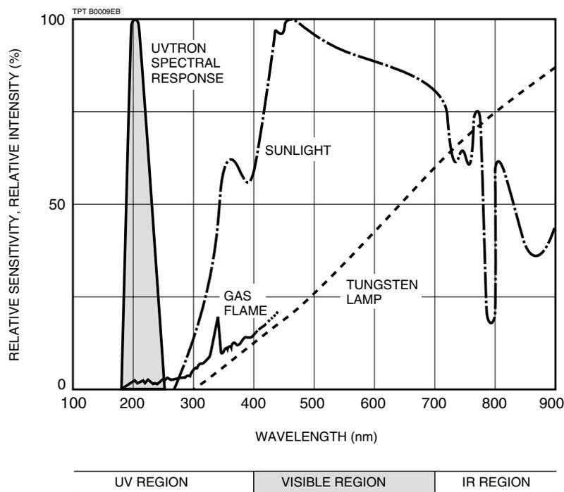
**Figure 1: Typical Spectral Radiant Intensity**
