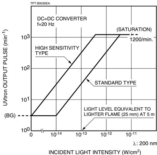
Figure 5: UVTRON Sensitivity and Background
