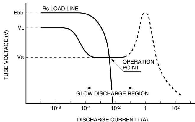
Figure 3: UVTRON Voltage-Current Characteristics
