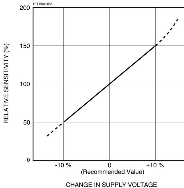
Figure 9: Supply Voltage and Sensitivity
