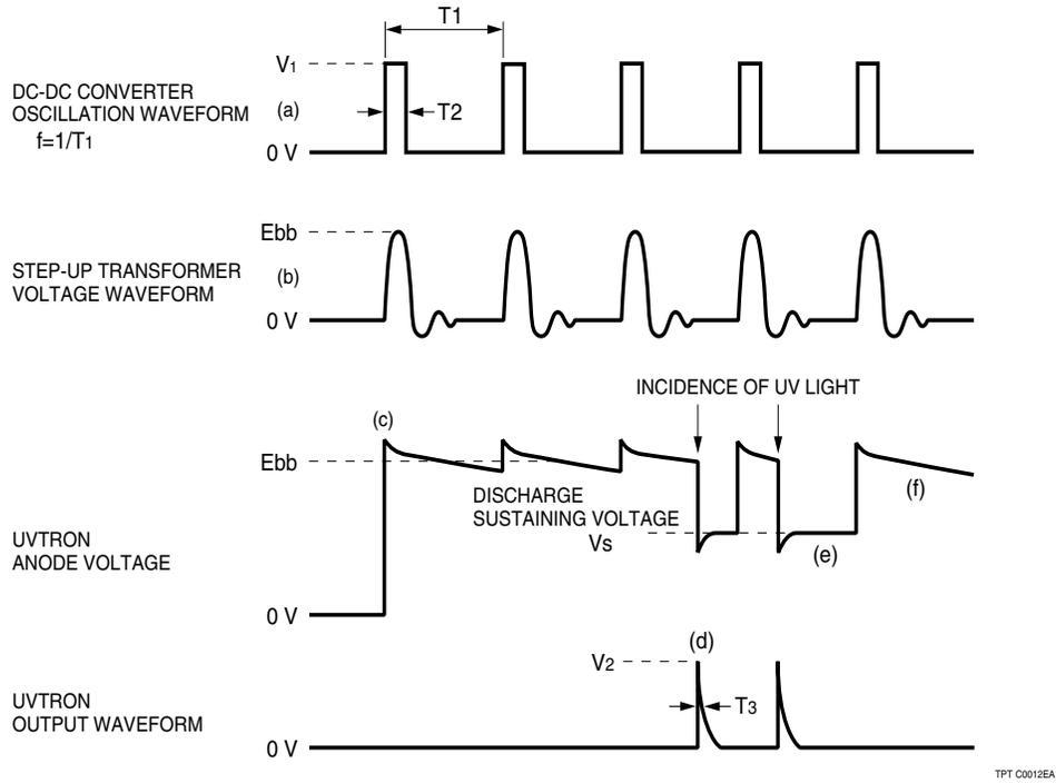
Figure 4-2: UVTRON Operation Waveforms
