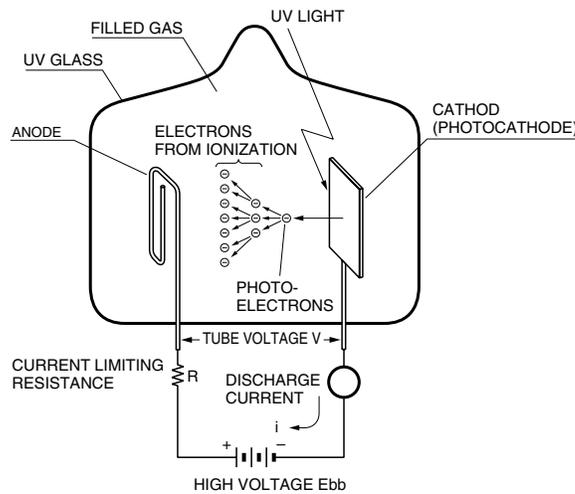
Figure 2: Schematic of UVTRON Operation
